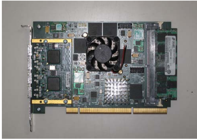
FPGA board H101-PCIXM manufactured by Nallatech.
