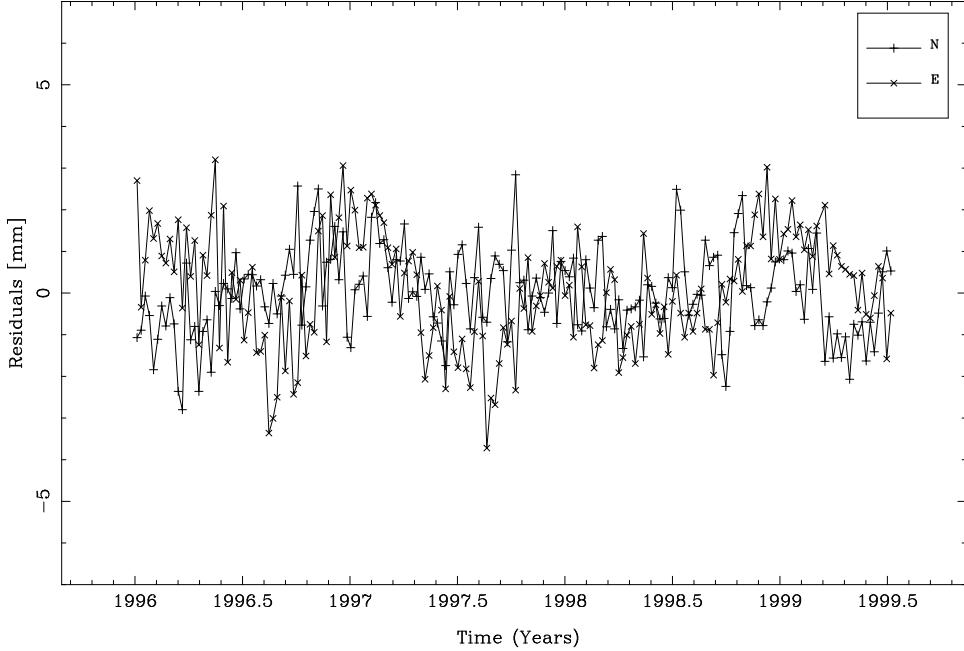
Figure 1: North and East residuals of weekly coordinate estimates with respect to the multi-year solution for site Kootwijk (KOSG), The Netherlands.
